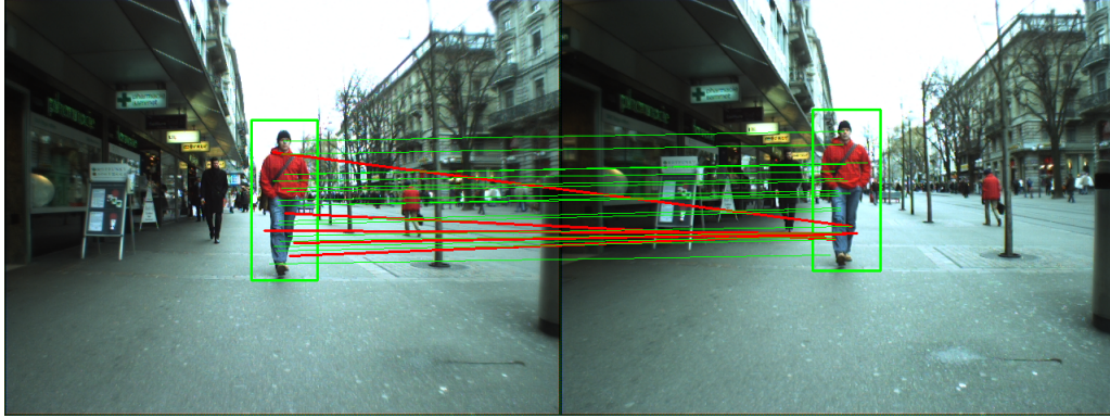
Figure 2. Pairs of correspondent points obtained with SURF. Red color is used to denote wrong matches or non-interesting correspondent points from background.
