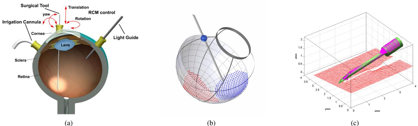
Figure 1: (a)The sub-retinal injection surgery which needs highly precision and delicate motion, (b)The needle placement on the surface of retina, and (c)The needle reconstruction using OCT image cube.
