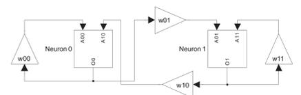
Figure 6: simple neuronal oscillator in MATLAB SIMULINK
