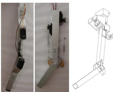
Figure 5: adaptive compliant mechanisms: Macepa (H<sup>+</sup>06) knee joint (left), antagonistic knee joint (center), concept of antagonistic knee joint with detachable spring (right)
