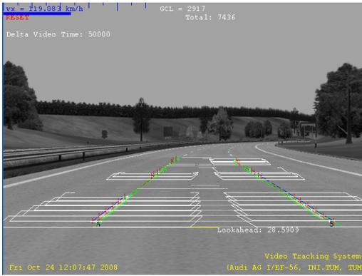
Figure 3. Lane tracker working on rendered synthetic image
