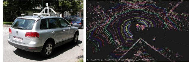
Fig. 2. 3D LIDAR scanner: (left) the experimental vehicle, (right) raw data from an urban scene.
