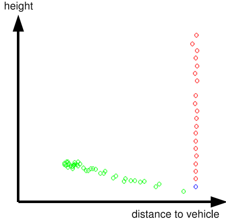
Fig. 4. Profile plot, points are classified into obstacle (red) and surface (green) points. Blue points are drivable road, lying behind obstacles. The height axis in the picture corresponds to the z-axis of the car’s coordinate-system, the distance axis points in a certain rotational direction.
