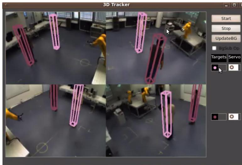
Figure 3.3: Graphical user interface for controlling the system and visualizing the tracking results
