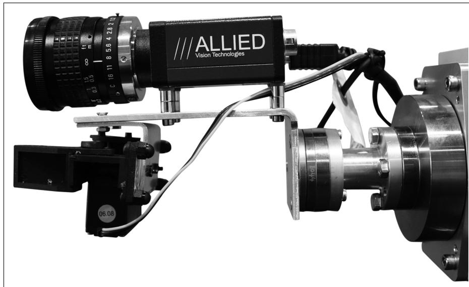
**Figure 4.2:** The custom made gripper construction
