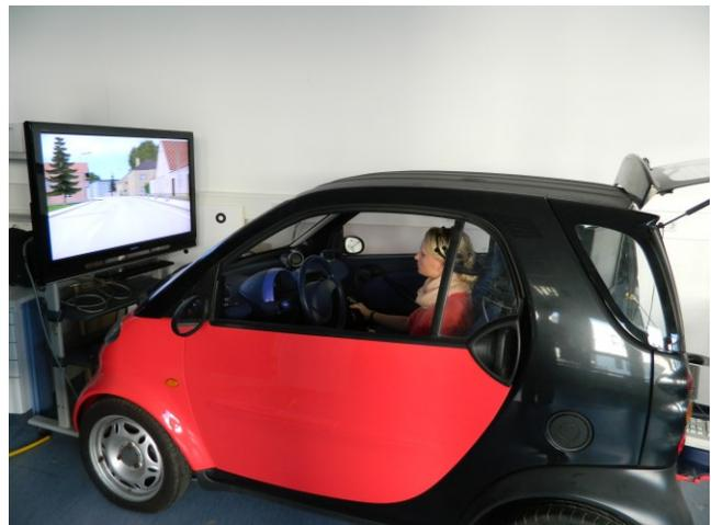
Figure 9. The driving simulator mock-up built upon VIRES Virtual Test Drive.
