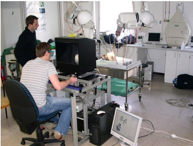
Fig. 1. **Hardware Setup:** Ceiling mounted robots with surgical instruments
