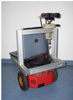
Fig. 8. The Pioneer3-DX carrying the two Marlin cameras.
