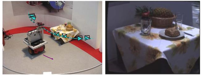
Fig. 5. (Left): Acquisition of a set of images with a stereo camera head mounted on a Pioneer 3-DX. (Right): A virtual image rendered from selected reference images. The virtual camera is placed at a position where there is no real camera.
