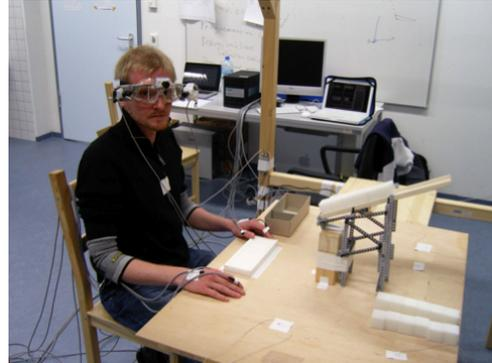
Fig. 1: **Baja experimental set-up** - Subjects assemble a tower by combining six cubes provided by a cube vendor in front of them with several bolts taken from a box on their left. During the experiment sensor record the position of the thumbs, the forefingers, the back of both hands, the head, the torso, and the gaze [4]
