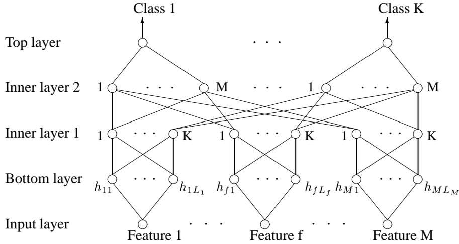
Figure 2: Structure of the neural network used in the AFRB.
