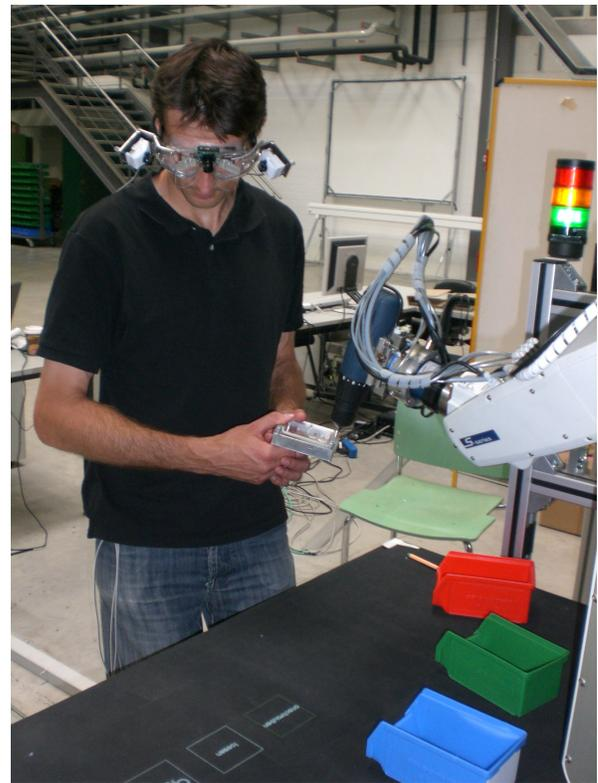
Fig. 3. Human worker and industrial robot in hybrid assembly.
