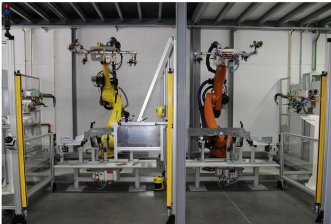
Fig. 1. Robotic Spot Welding Cells at Introsys
