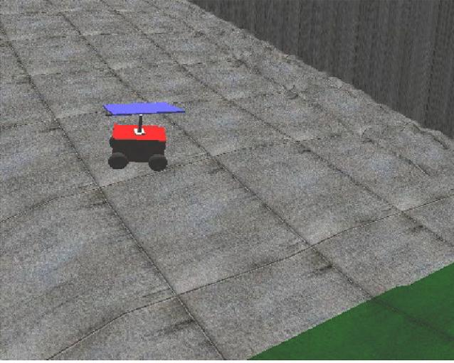
Fig. 8. The robot has succeeded in leveling the platform. The roll, pitch, yaw of the robot is still (-23.2, -3.5, 65.5) but that of the platform is (-0.8, -1.5, -14.4). A tolerance of  $\pm 1.7$  degrees deviation from zero was allowed.
