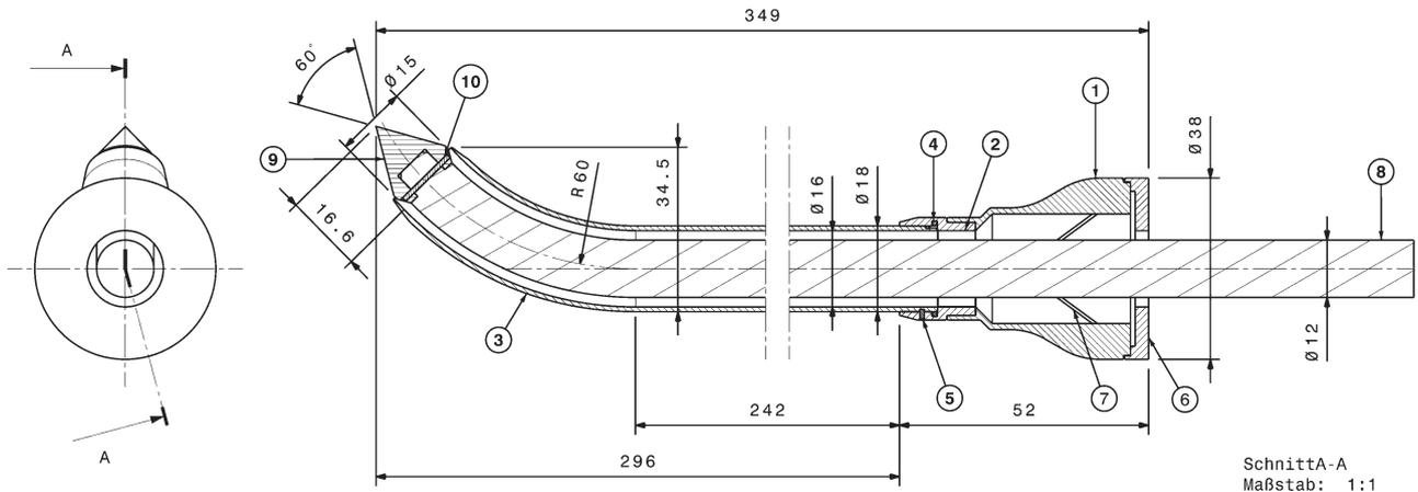
Figure 1. Cross-section of the ISSA trocar with inserted part flexible obturator; (1) trocar head, (2) trocar adapter, (3) trocar tube, (4) O-ring seal, (5) bayonet mechanism, (6) front cap, (7) trocar valve, (8) part flexible obturator, (9) conic front end, and (10) pin.
