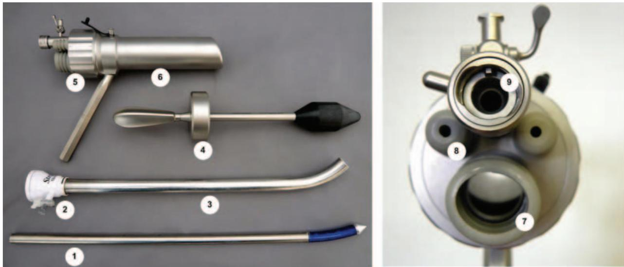
Figure 3. The new set of instruments (ISSA) designed to permit sterile sigmoid access for transcolonic surgery; (1) part flexible obturator, (2) trocar head, (3) trocar tube, (4) TEM obturator, (5) modified TEM cap, (6) modified rectoscope, (7) trocar port, (8) instrument ports, and (9) optical port.
